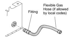
Figure 11 - Attaching Flexible Gas Hose to Heater
